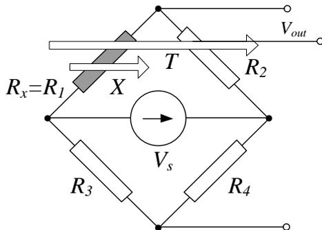
FIGURE 2.31 The bridge circuit a tool to apply the differential principle.
