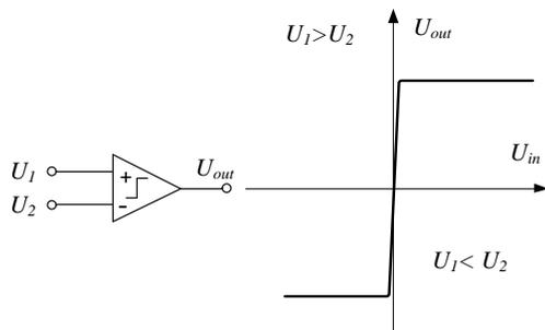
FIGURE 2.4 The principle of operation of the comparator.
