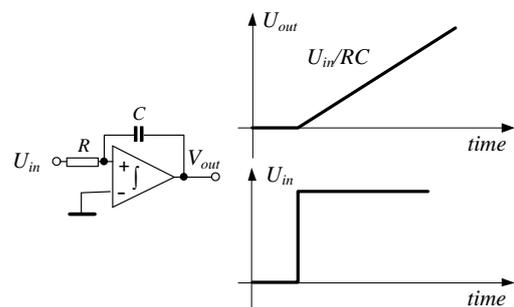
FIGURE 2.6 The integrating amplifier as the source of linearly increasing voltage.
