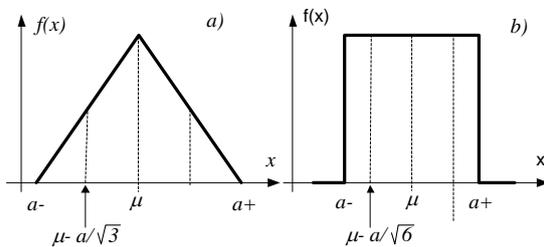
**FIGURE 2.48** The graph of the triangular (a) and rectangular (b) density of probability function. There are indicated the range of variable corresponding with standard deviation  $3\sigma$  of normal distribution
