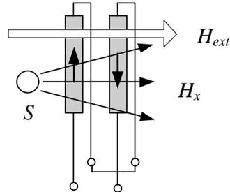
FIGURE 2.33 Two differential sensors used as a gradiometer.
