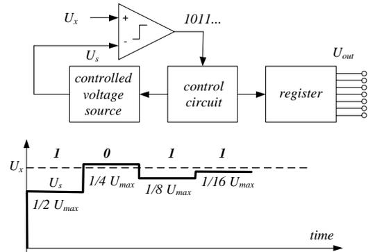
FIGURE 2.5 The digital compensation device - SAR.
