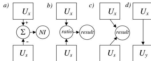
**FIGURE 2.1** Various methods of comparison of two values: a) compensation, b) comparator, c) substitution, d) conversion.
